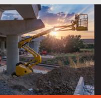
Remember: The catapult effect can also occur when driving in the stowed position, so make sure occupants wear personal fall protection equipment (PFPE) connected to the designated anchor point at all times. Occupants must always use a full body harness and an adjustable restraint lanyard, adjusted as short as possible, when using boom-type MEWPs.
