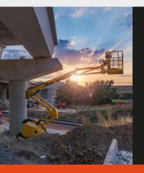
Remember: The catapult effect can also occur when driving in the stowed position, so make sure occupants wear personal fall protection equipment (PFPE) connected to the designated anchor point at all times. Occupants must always use a full body harness and an adjustable restraint lanyard, adjusted as short as possible, when using boom-type MEWPs.
