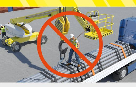
Mobile elevating work platforms (MEWPs) are designed to lift people to a position where they can work at height safely in the platform. MEWPs are not designed to be used as an overhead anchor point. Using them as such is **not recommended**.
