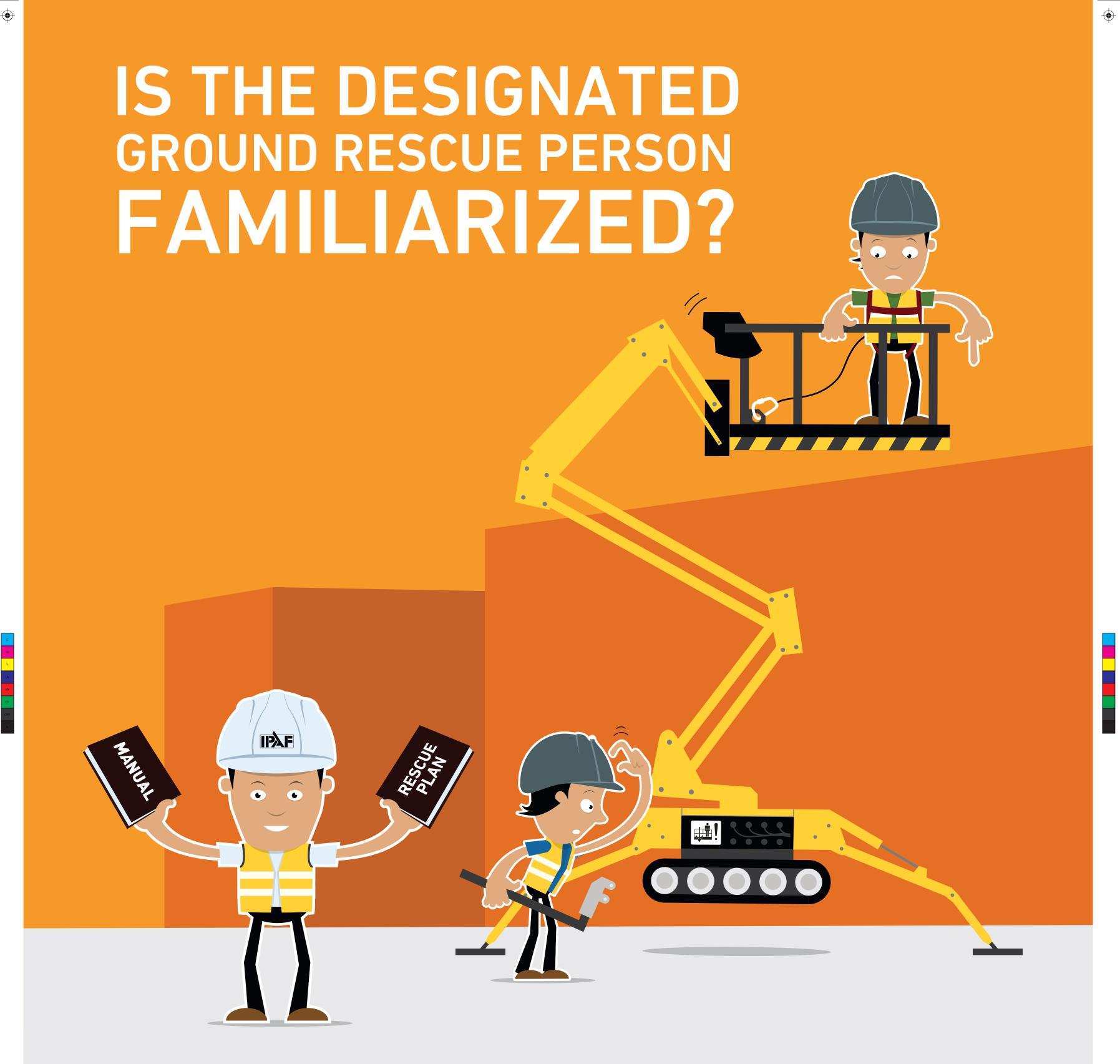
MEWP MODELS ARE DIFFERENT. LEARN AND PRACTICE THE GROUND CONTROLS AND THE AUXILIARY/EMERGENCY LOWERING CONTROLS AND PROCEDURES ON YOUR MACHINE.
