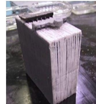
AGM plate/separator stack after compression
