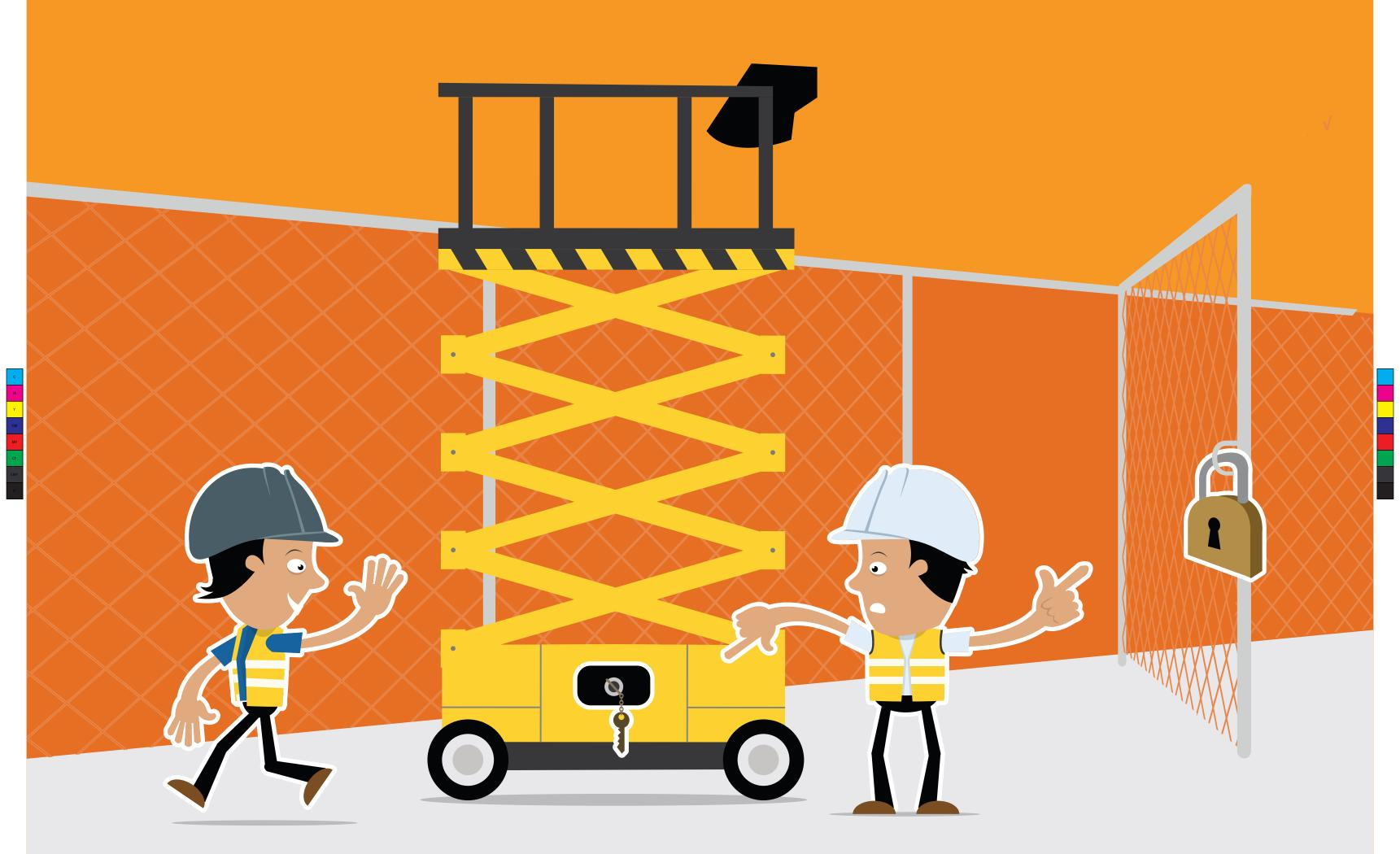
AFTER USE, ALWAYS LEAVE THE MACHINE IN A SAFE AND SECURE PLACE AND REMOVE THE KEY
