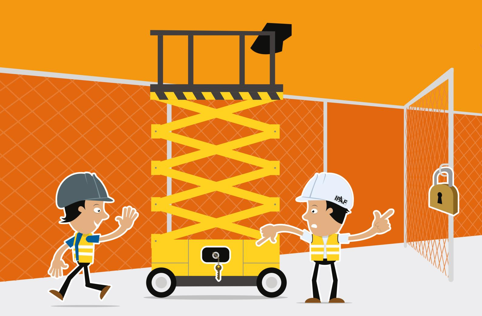
AFTER USE, ALWAYS LEAVE THE MACHINE IN A SAFE AND SECURE PLACE AND REMOVE THE KEY
