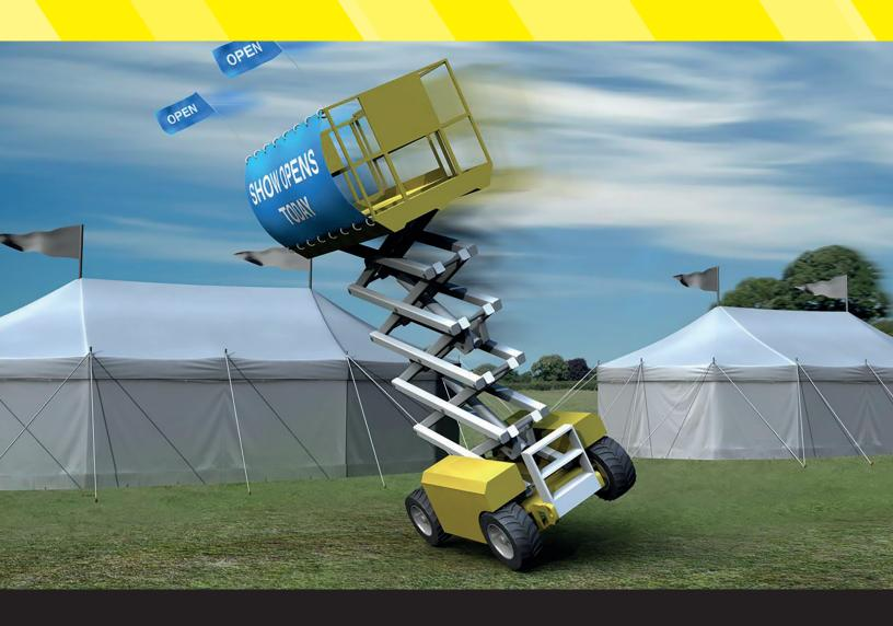
Many scissor lifts are specifically designed for indoor use only with zero wind. Even outdoor machines may be at risk of being blown over when elevated in high or gusting winds.
