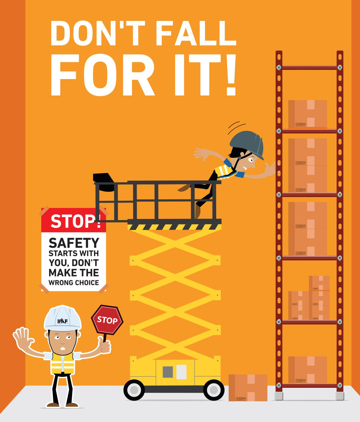
POSITION YOUR MEWP CORRECTLY AND ALWAYS STAY INSIDE THE PLATFORM GUARDRAILS WITH BOTH FEET ON THE PLATFORM FLOOR
