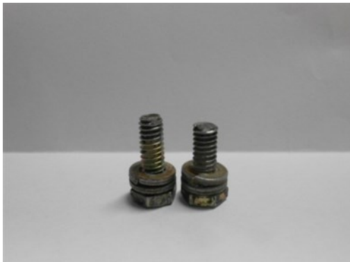
ORIGINAL BOLT LENGTH ON THE LEFT, WORN BOLT ON THE RIGHT
