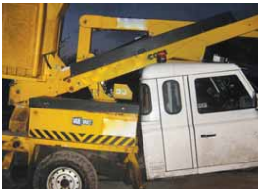
The chassis failure with the rear radius arm fixing to the bottom right
